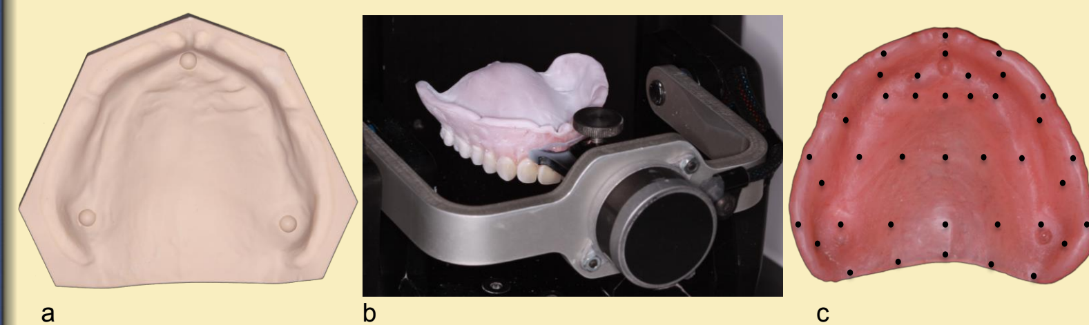
Figure 1. (a) Maxillary master cast (b) Denture in scanner (c) 40 measuring points
