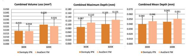
**Figure 6:** Combined Wear Results. Upper and lower values for a wear parameter were combined to give the total wear for the two materials. There were no statistical differences between Dentsply IPN and AvaDent FM. The number of samples for Dentsply IPN and AvaDent FM were 4 and 5, respectively. The error bars represent one standard deviation.
