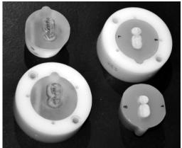
Figure 3a: Test samples with mounting rings AvaDent FM samples are clear; Dentsply IPN samples are white.
