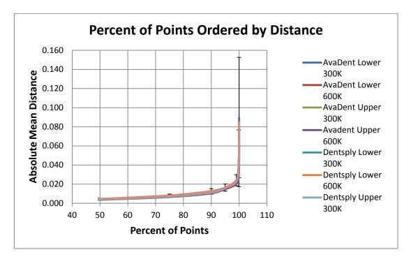
**Figure 7:** Quality of alignment of digital model. All alignments are to the baseline model. The error bars are the largest standard deviation of the eight comparisons for a given percentage.
